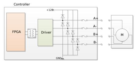
Picture 10 Connection of throttle step motor
