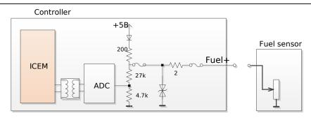
Picture 11 Connection of fuel level sensor
