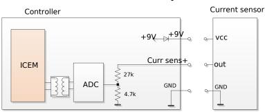
Picture 12 Connection of generator current sensor
