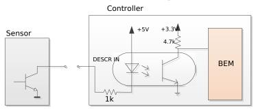
Picture 13 Open collector output and discrete input
