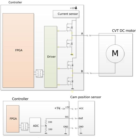
Picture 7 Connecting of CVT DC motor and cam position sensor
