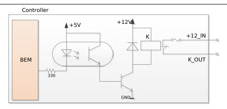
Picture 14 Connection of board equipment to the controller relay
