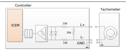
Picture 8 Connection of IC engine tachometer
