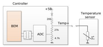
Picture 9 Connection of resistive temperature sensor
